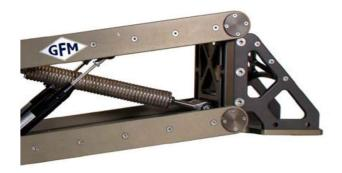
To change from over to under slung, remove the 3 bolts on the underside of the Mitchell plate and the 3 bolts on each side of the Mitchell mount.
