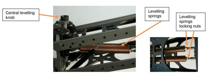
Turning the central levelling knob clockwise will raise the arm, anticlockwise will lower it.
