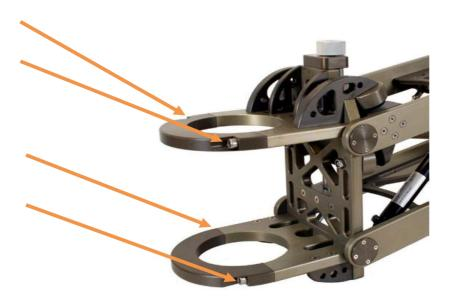
Connect the Maxi SA to the respective tube and secure by clamping it in the required position and tightening the 4 locking bolts.
