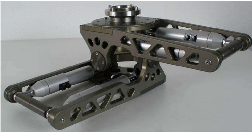
The Iso Dampener increases the efficiency of gyro stabilized heads by reducing rotational stress and smoothing out pan starts and stops on telescopic and fixed arm cranes by isolating high frequency vibrations between the mount and head.
